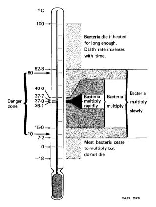
Fig. 3. Control of pathogenic bacteria by temperature.
